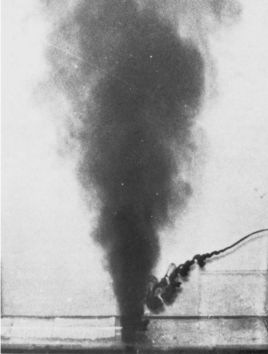
FIGURE 20. Medium time exposure (2 s) photograph of a turbulent two-dimensional jet ( Re \approx 2500, R_0 = 0 ).
