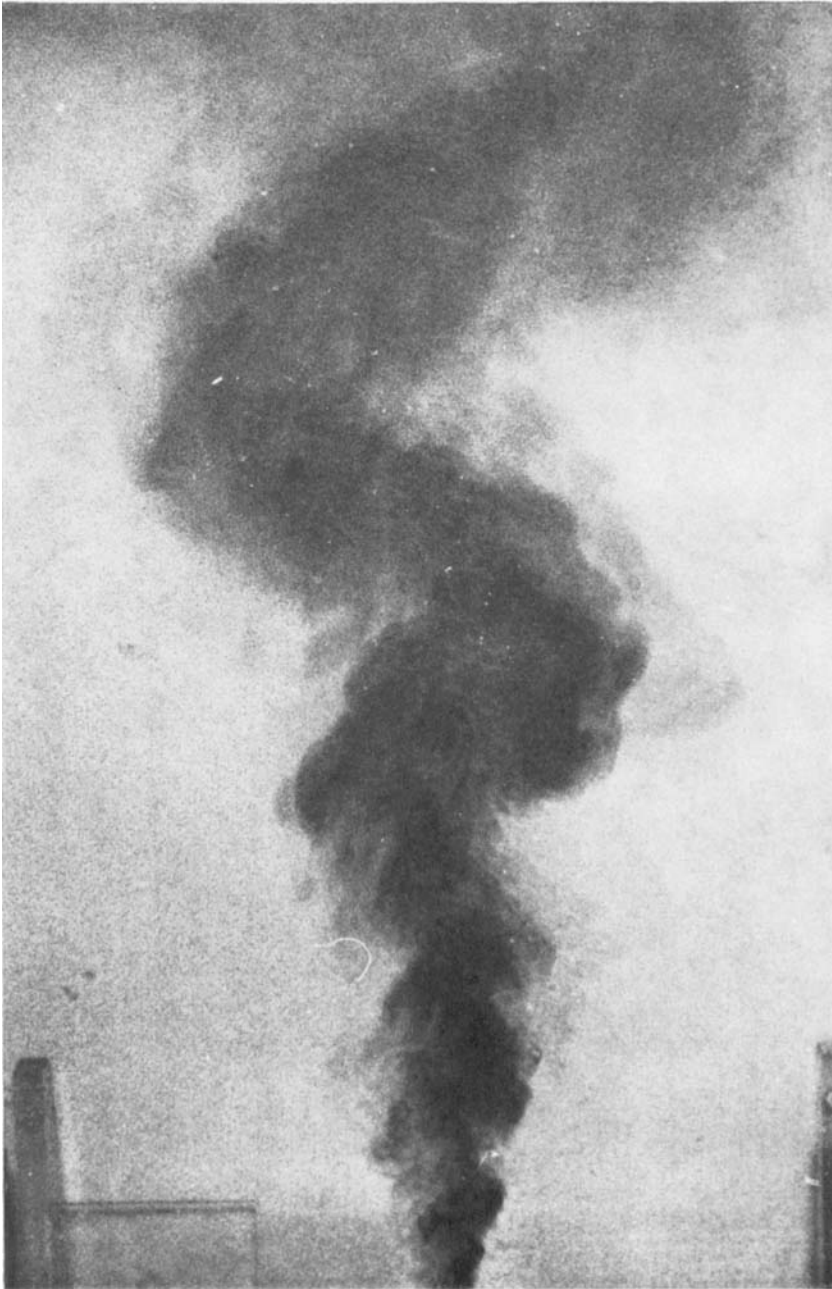
FIGURE 18. Short time exposure (0.01 s) photograph of a turbulent two-dimensional plume ( R_0 \approx 0.5 ).
